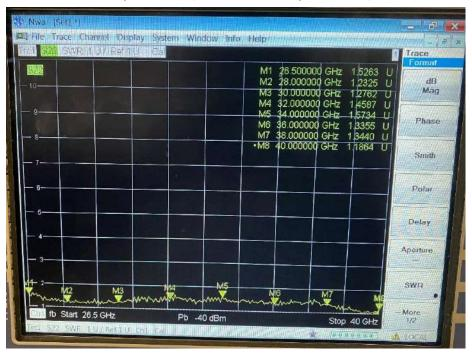
Output VSWR @ Pin=-40 dBm (Ambient temp. +25±3 °C, DC Voltage= 22V)
