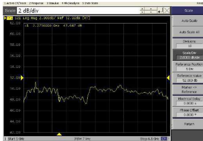
Graph4: Power Gain@ Pin= 0 dBm: (Ambient temp. +25±3 °C, DC Voltage= 28V, Load VSWR ≤ 1.2)
