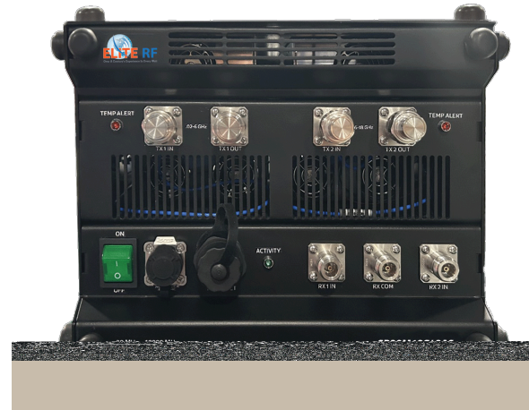
Wideband 20MHz to 18GHz RF Amplifier for military application
