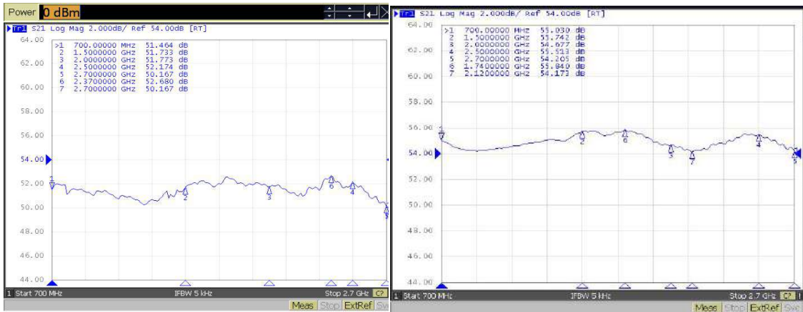
Figure left: Input Return Loss S11 ( [Pin=-30dBm, CW, Load VSWR≤1.2, 25°C]
